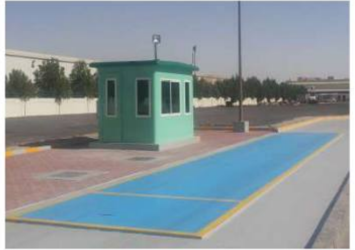
PIT TYPE WEIGHBRIDGE
